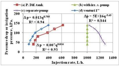
Fig. 5: Hydraulic characteristics of chemical injector equipment.
