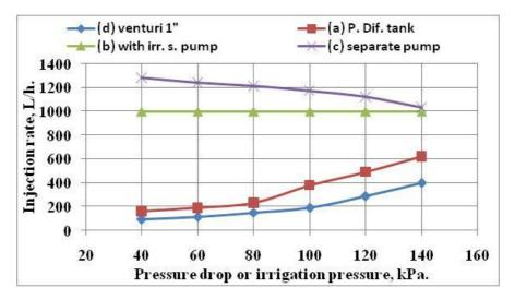
Fig. 2 : Performance of chemical injectors.
