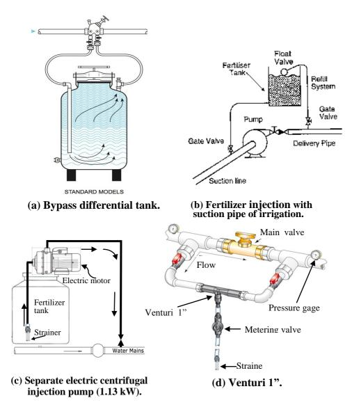
Fig. 1. Chemical injection equipment.
