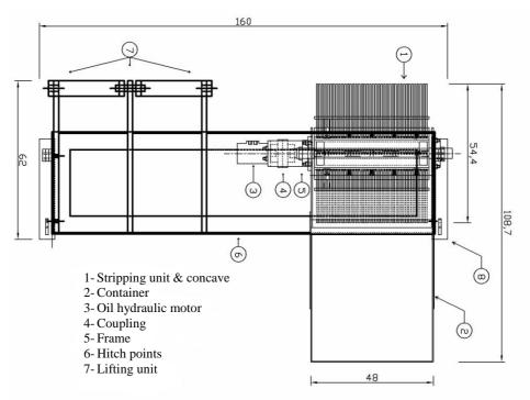
Fig. 5. Plan of the 1<sup>st</sup> snap bean stripping prototype
