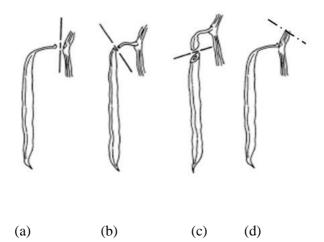
Fig. 4. Failure types of the pod-pedicel-stem structure
