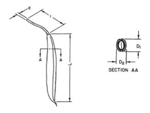
Note: dimensions  $d_1$  and  $d_2$  taken at three positions along length of pod; mean recorded.
