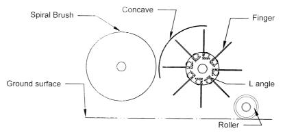
Fig. 7. Side view of spiral brush reel fingers as a stripping unit
