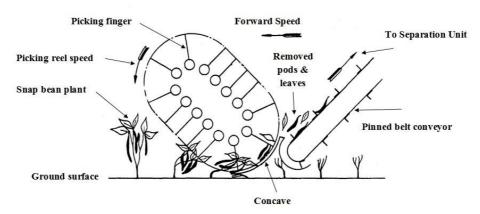
Fig. 6. Conveying band and reel fingers as a deflection unit
