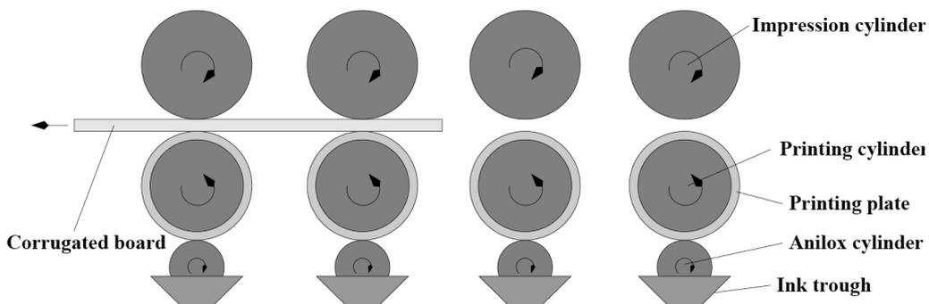
**Figure 1:** Shows A flexo printing press with four printing stations.
