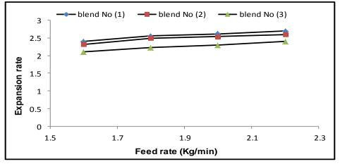
Fig. 4. Effect of feeding rate on expansion rate of extrudates.
