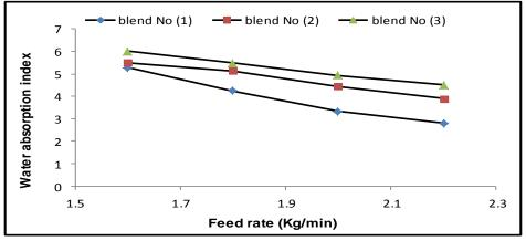
Fig.10. Effect of feeding rate on water absorption index of extrudates.
