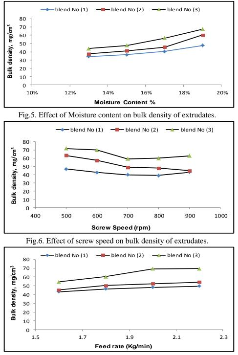
Fig.7. Effect of feeding rate on bulk density of extrudates.
