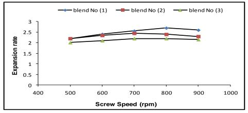
Fig. 3. Effect of screw speed on expansion rate of extrudates.
