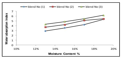
Fig.8. Effect of moisture content on water absorption index of extrudates.
