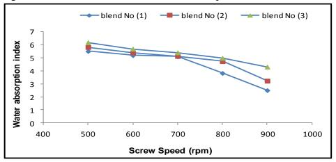
Fig.9. Effect of screw speed on water absorption index of extrudates.
