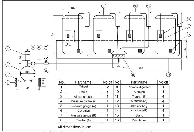
Fig. (1): Diagram of the compost tea production unit.
