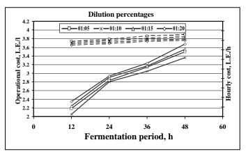
Fig. (4): Effect of temperature degree, air pressure and fermentation period on hourly and operational costs at different dilution percentages.
