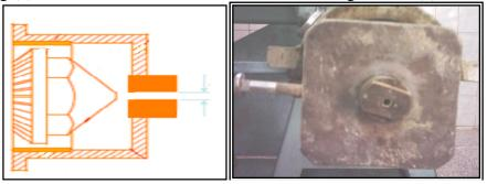
Fig. 4. The parts and a photo for the extruder's die area and the die.
