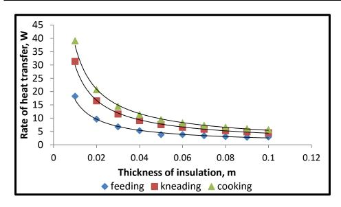
Fig .2. The rate of heat transfer from the insulated barrel to the surrounding air.
