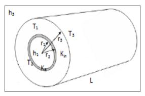
Fig. 1. The insulation cylindrical pipe surrounding the extruder barrel.
