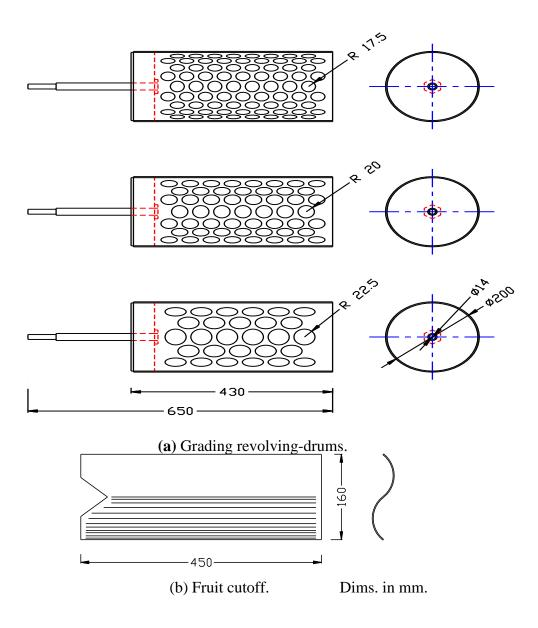
Fig. 3: Views of grading revolving-drums and fruit cutoff.
