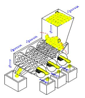
Fig. 5 : Schematic diagram of the designed grading-machine, with the numbers in brackets indicating parameters necessary for design of different parts.
