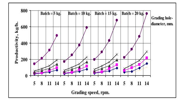
**Fig. 9:** Effect of grading speed, hole diameter of grading drums and fruit batch on machine grading-productivity.
