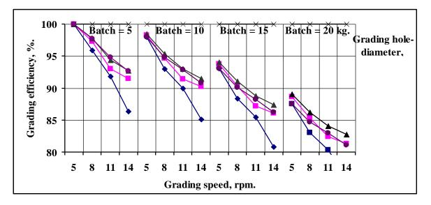
**Fig 9 :** Effect of grading speed, hole diameter of grading drums and fruit batch on machine grading-efficiency.
