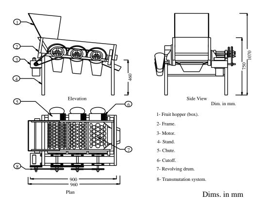
Fig. 1: Views of designed grading-machine for lemon fruits.
