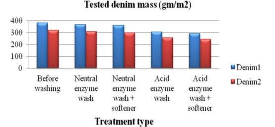
Fig.4: Tested denim mass before washing, after washing and after softening
