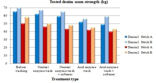
Fig.9: Tested denim seam strength before washing, after washing and after softening
