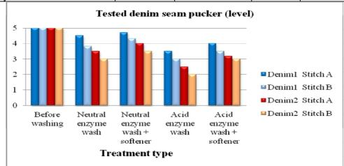
Fig.10: Tested denim seam pucker before washing, after washing and after softening
