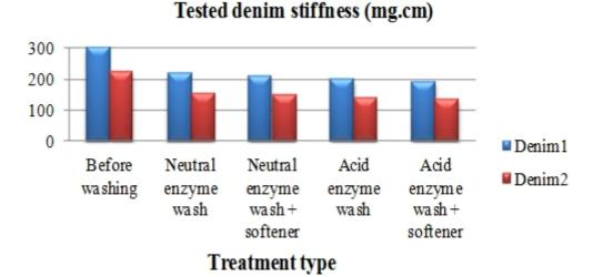
Fig.7: Tested denim stiffness before washing, after washing and after softening
