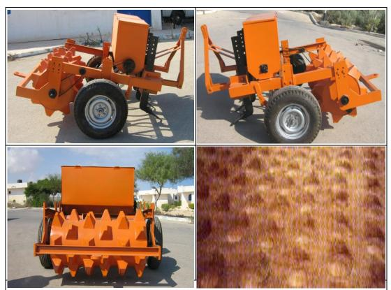
Fig. (2): Photos of the developed combination unit and the experimental area with the mini reservoirs made by the machine.
