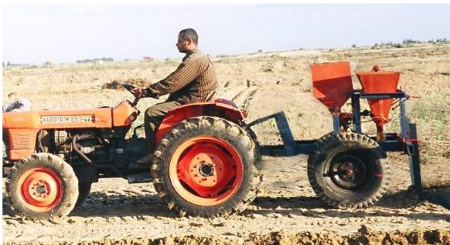
Fig. 1-B: The photograph of fertilizer prototype Fig. 1: The prototype of Fertilizer
