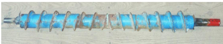
Fig. 2-B: The fertilizing auger shaft
