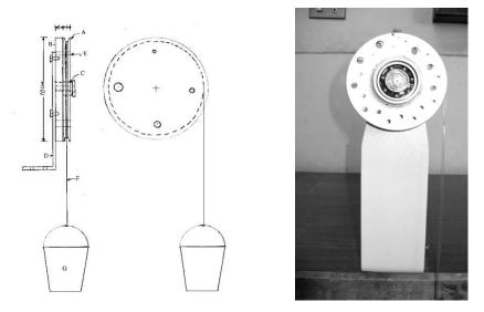
Figure (1): Static Shear CellApparatus.(A-Moving Disc B- Fixed Disc C- Ball Bearing D- HolderE- HoleF- Rope G- Water Bucket)
