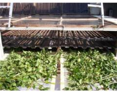
Fig. 4. Fresh Peppermint put over tray to dry in the solar dryer
