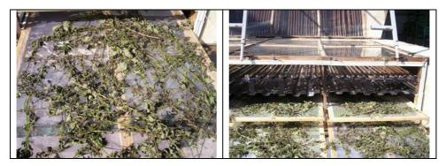
Fig. 7. Dried Lemon Balm put over tray in the solar dryer
