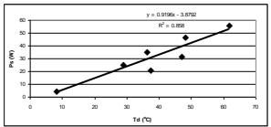
Figures (11): The standardized cooking power as a function of temperature difference (Tw-Tamb) for aluminum box with 1 kg of water.
