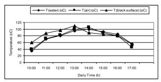
Figures (5): Effect of Cooker Type on the Cooker Temperatures for carton box with 1.0 kg of water
