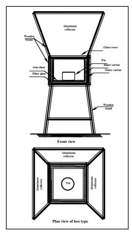
Figure (1) Front and plan view of carton cooker
