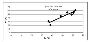
Figures (9): The standardized cooking power as a function of temperature difference  $(T_w-T_{amb})$  for carton box with 1 kg of water.
