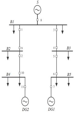
Fig.3 Single line diagram of the tested distribution system
