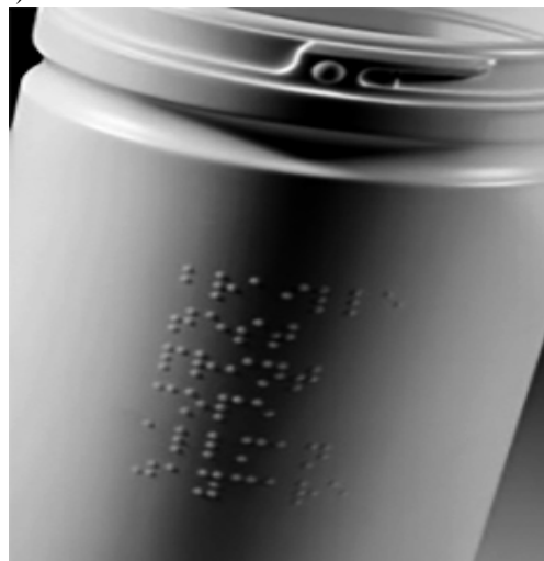
Figure (5): Braille text printed with UV ink on a plastic bottle by screen printing
