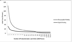
Figure (2): Cost comparative between digital and Flexographic printing systems.
