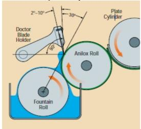
Figure 1: Flexographic Printing Process<sup>(5)</sup>.
