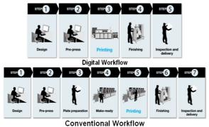
Figure (3): Comparison between Digital and Conventional Workflow<sup>(13)</sup>.
