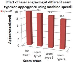
Fig.7. Effect of laser engraving at different seam types on appearance using machine speed1 Effect of laser engraving at different seam types on
