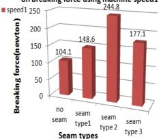
Fig.3. Effect of laser engraving at different seam types on breaking force using machine speed1
