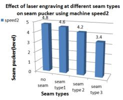
Fig.6. Effect of laser engraving at different seam types on seam pucker using machine speed2
