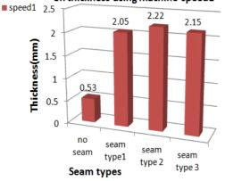
Fig.1. Effect of laser engraving at different seam types on thickness using machine speed1
