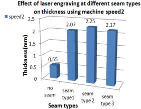
Fig.2. Effect of laser engraving at different seam types on thickness using machine speed2
