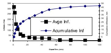
Fig. 2: Infiltration and cumulative for tested irrigation border.
