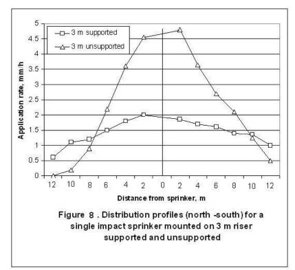
Which allowing sprinkler vibration, inclined from the vertical, thereby effectively increasing the trajectory angle. It may be concluded that well-supported risers made from steel pipe lead to very little vibration. Plastic pipe could be used as riser material, but it is more flexible and will undergo more vibration. To minimize riser vibration interference with sprinkler operation, plastic risers need to be rigidly supported.
