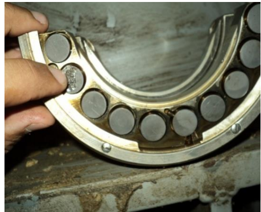
Fig.11. Defects at the thrust bearing pads
