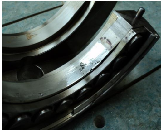
Fig.10. Defects at thrust bearing 2nd half inner angular race
