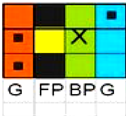
Fig 4. The weave repeat of the terry fabric (Basic 3-pick terry weave in 2:2 warp order) [25]
