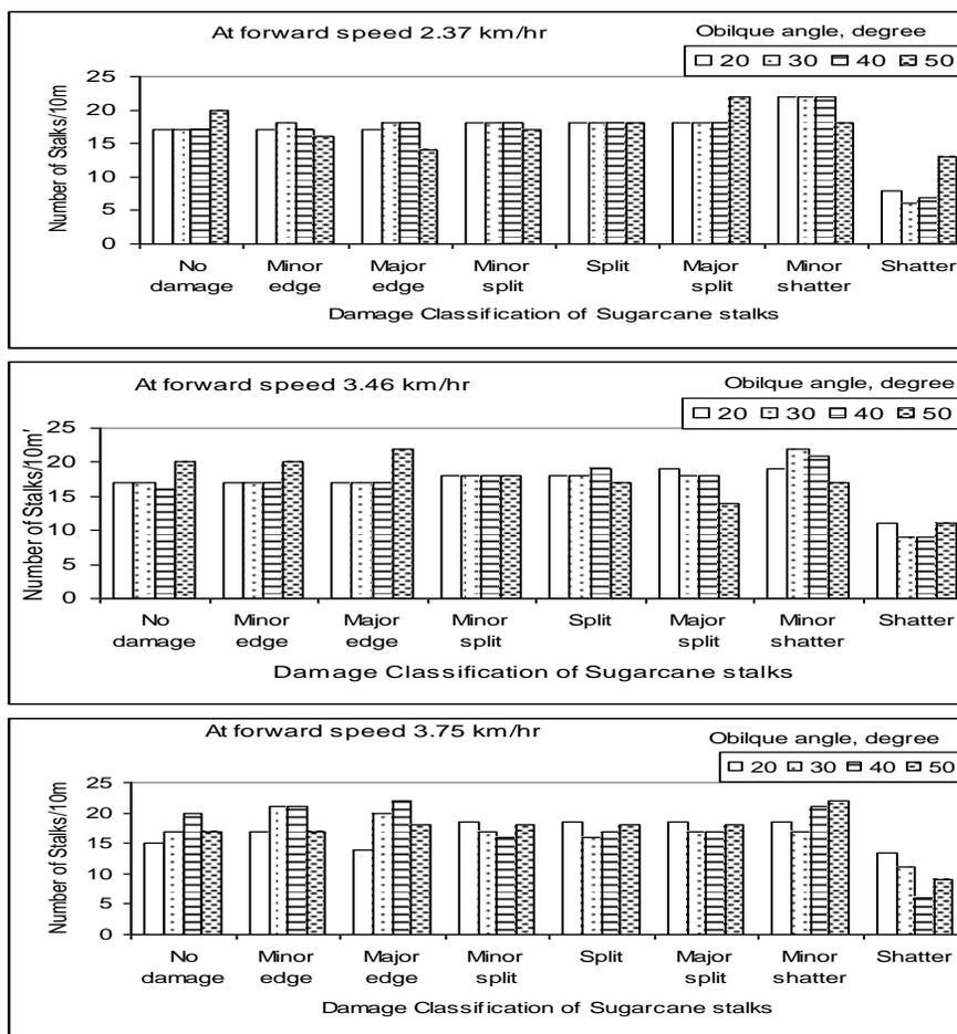
Fig. (8) Effect of forward speed on damage classification of sugarcane stalks
