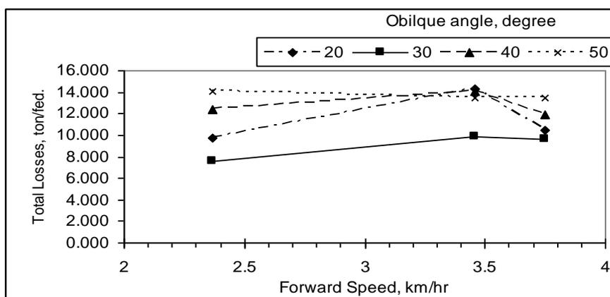
Fig. (7) Effect of forward speed on total losses
