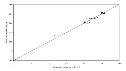
Fig. 5: The goodness of drawbar pull predicting by equation for moldboard plow.
