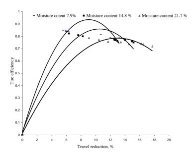
Fig. 2: Effect of soil moisture content and travel reduction on tire efficiency for chisel plow
