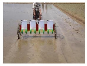
Fig (1) Photograph of a developed direct seeding rice machine
