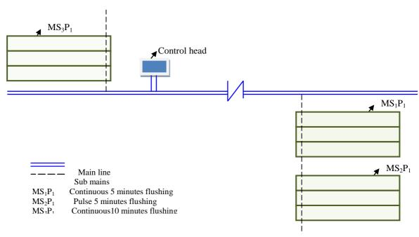
Fig.1:Flushing with water programs location.
