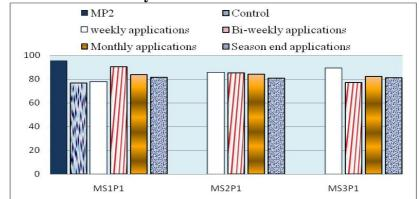
Fig.2.Effect of flushing programs on Distribution uniformity discharge criteria.
