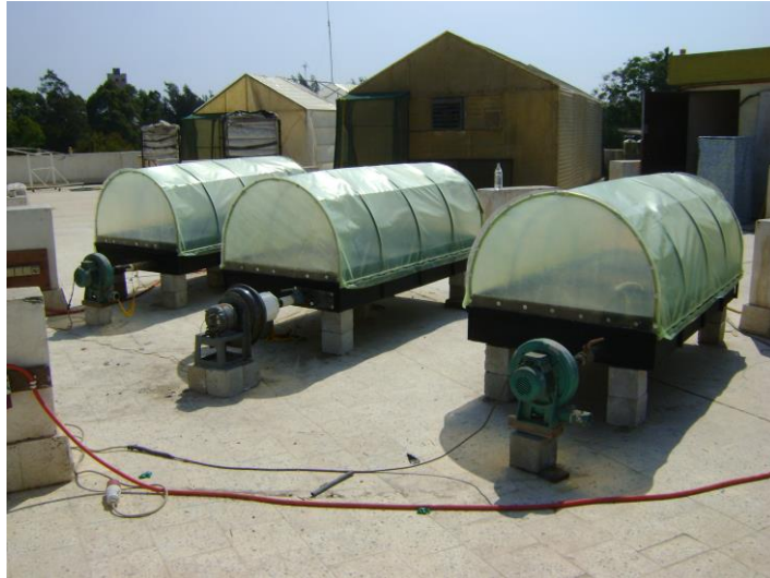
Fig. (1): Solar tunnel greenhouses (Quonset type) using as an active solar dryers during the experimental period.
