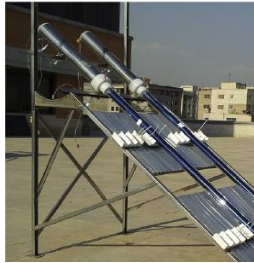
condenser mounted axially above with evacuated tube condenser [4]
