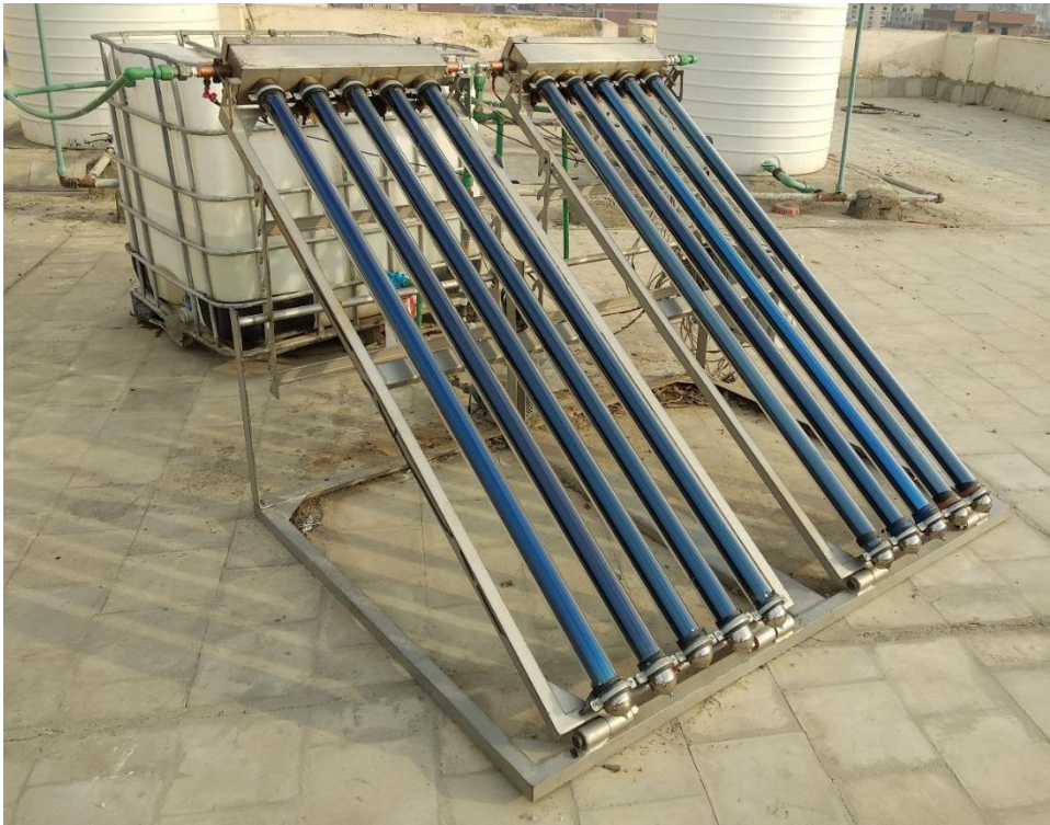
Figure 3. Photograph showing constructed test rig with two independent collectors
