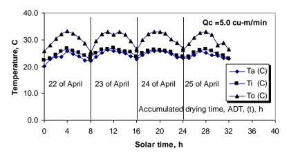
**Fig. (7):** Ambient air temperature (Ta), °C, inlet solar collector air temperature (Ti), °C and outlet solar collector air temperature (To), °C, versus accumulated drying time (t), Hr and solar time with active solar drying system through a solar air collector airflow rate Qc =5.0 cu-m/min.
