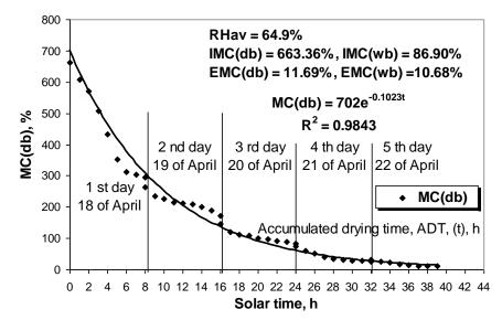
Fig. (3): Moisture content dry basis, MC(db), % versus accumulated drying time (t), h and solar time at natural sun drying system of marigold petals.
