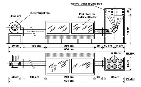
Fig. (2): Active solar drying system.
