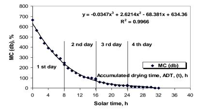
**Fig. (6):** Moisture content dry basis, MC (db), %, versus accumulated drying time (t), h and solar time with active solar drying system for marigold petals through a solar air collector airflow rate Qc=5.0 cu-m/min and active solar drying bed air flow rate Qb=1.250 cu-m/min.
