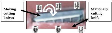
Fig. 2c: The fixed of chopping knives (after modification)
