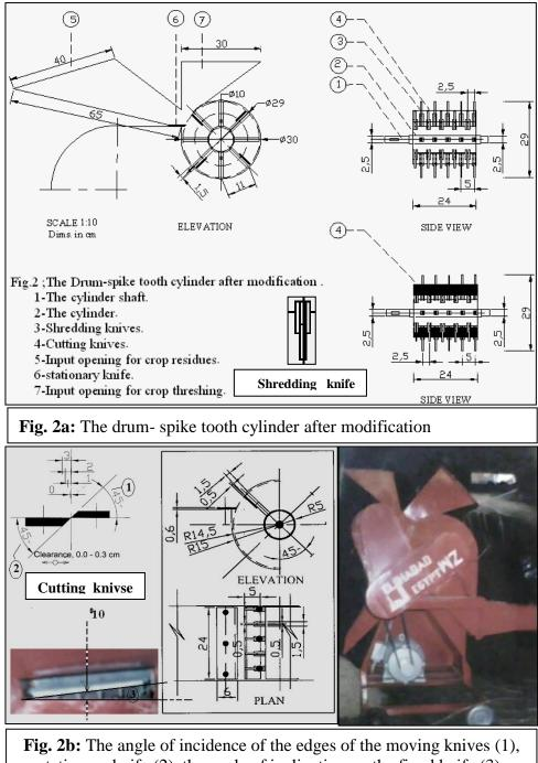
**Fig. 2b:** The angle of incidence of the edges of the moving knives (1), stationary knife (2), the angle of inclination on the fixed knife (3), diminutions and the machine after modification
