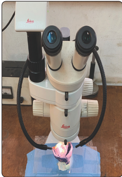
Fig. (7) Polyether impression analysis under the stereomicroscope and photographing with an attached camera of \times 60 magnification power.
