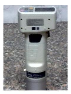
Fig. (2): Croma meter used to measure meat color samples by the CIE L, a, and b color system.
