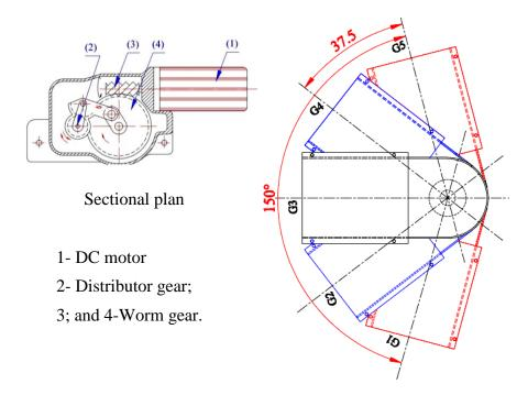
Fig. (4): Schematic diagram of distributing motor and position angle
