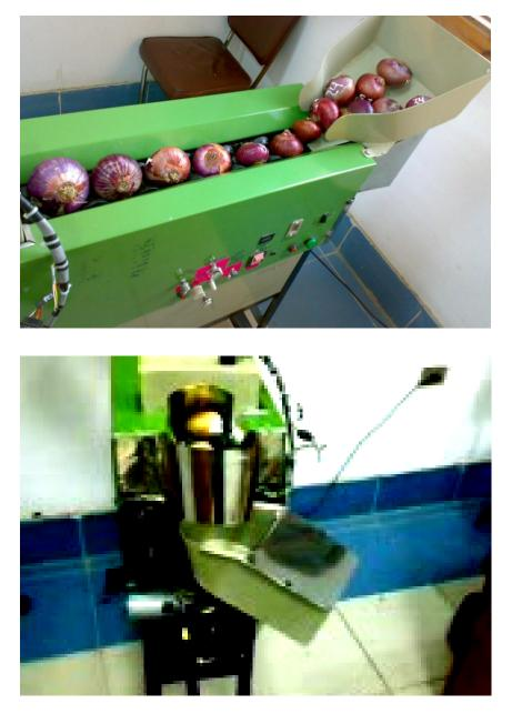
Fig. (2): Image of grading prototype (distributing motors).
