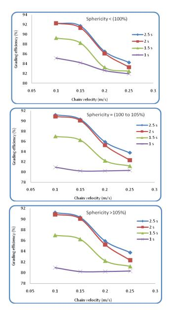
Fig. (8): Effect of conveyor chain velocity on the grading efficiency at different values of stopping time and sphericity percentage for onion.
