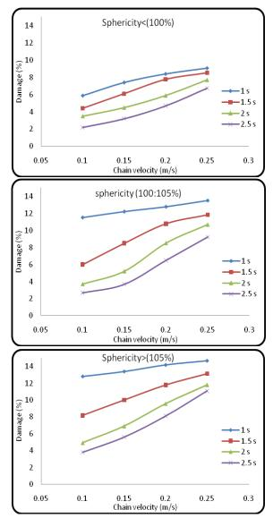
Fig. (9): Effect of chain velocity on damage percentage efficiency at different value of stopping time and sphericity percentage for onion.
