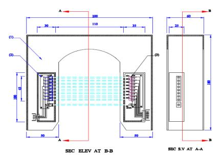
1-Housing, 2-Array of light emitting diode, 3-Array of optical sensor
