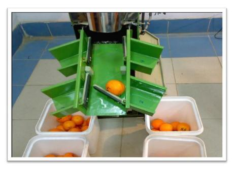
Fig. (2): Image of grading prototype (distributing gates)
