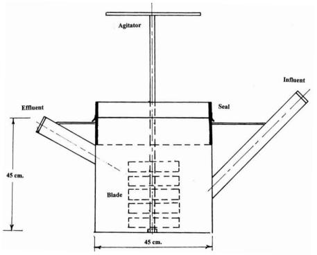
Fig.(1): The used digester, (Drawn to scale).
