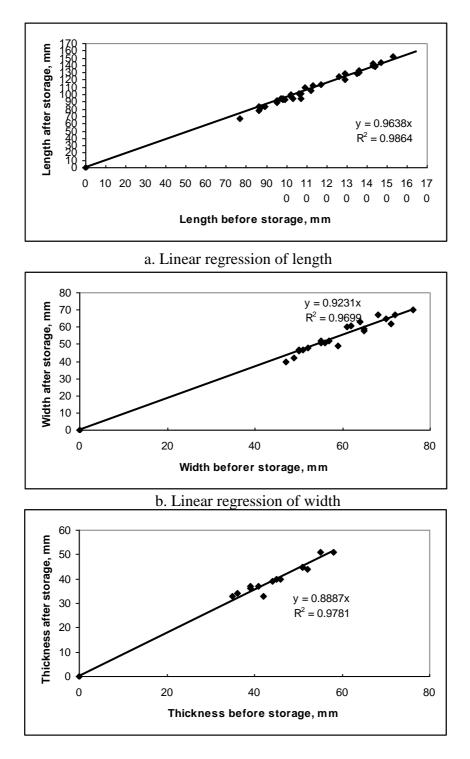
c. Linear regression of thickness Fig. 3: (, a, b, c): Linear regression of dimensions before and after storage.
