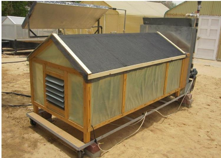
**Fig. (1): Experimental gable-even-span greenhouse**
