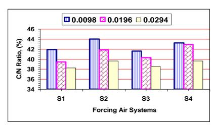
Figure 6. Effect of forcing air systems on carbon to nitrogen ratio of produced compost at different flow rates.
