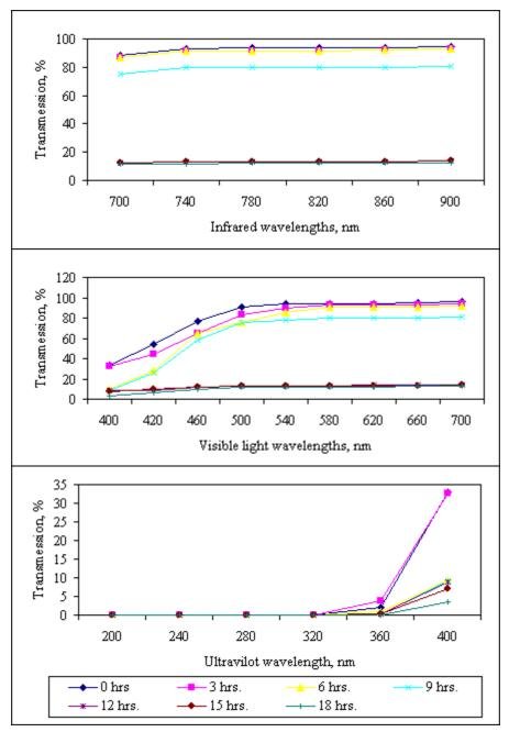
relationship between transmission and absorption light percentages from oil at different wavelengths.
