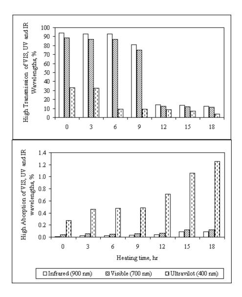
Fig. (4): High transmission and absorption light percentages through heated corn oil at wavelengths of Ultraviolet , Visible and Infrared .
