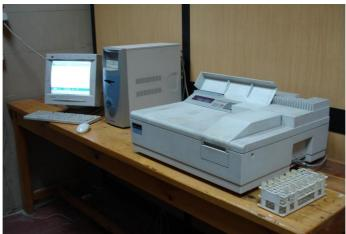
(b): Photo of spectrophotometer. Fig. (1): Diagram of double beam and photo of spectrophotometer.
