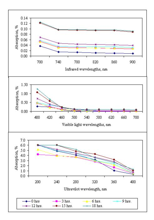
Fig. (3): Absorption light percentages from heated corn oil at different wavelengths.
