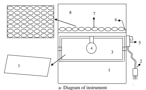
1- light box, 2- Electric source, 3- mirror, 4- light source, 5- switch, 6- screen, 7- milled rice grains, and 8- vision box.
