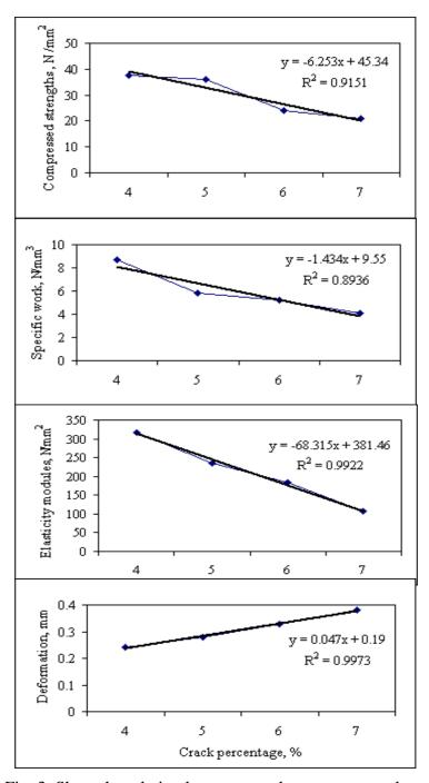
Fig. 3: Show the relation between crack percentage and some mechanical parameter of rice grains.
