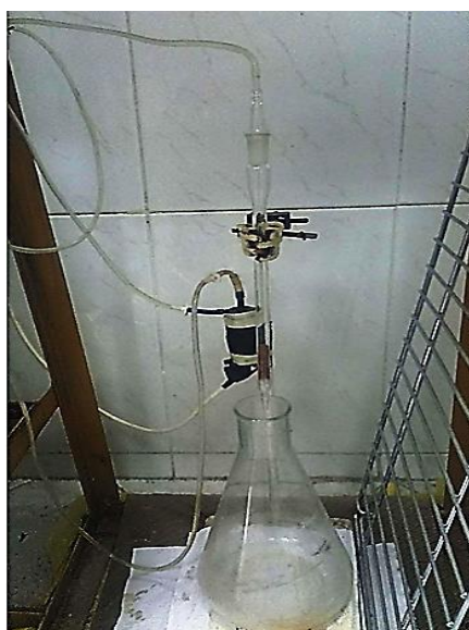
Fig. 2: Fixed-bed column set-up.
