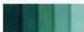
Samples of the glass olivaceous and turquoise color degrees from cobalt and chrome of the Research subject ( Co_2O_3 ), ( Cr_2O_3 )
