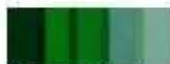
Samples of the glass green color degrees from chrome of the Research subject ( Cr_2O_3 )
