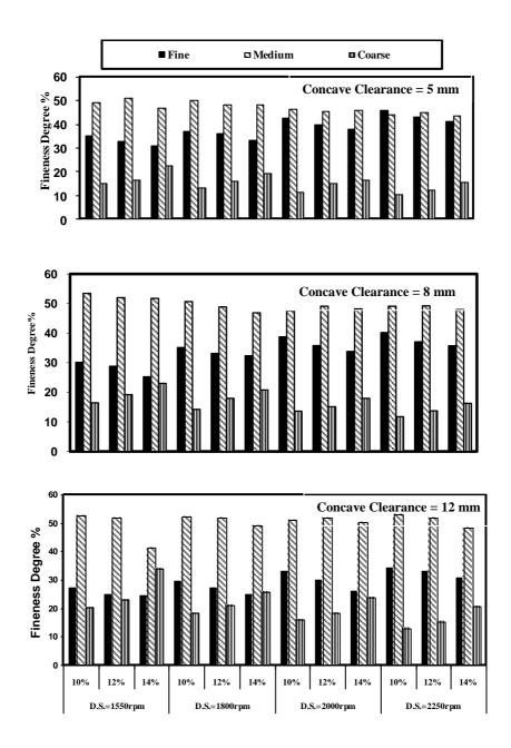
Fig.(6):Effect of drum speed on fineness degree under different moisture contents and concave clearances at hammer thickness of 3mm.
