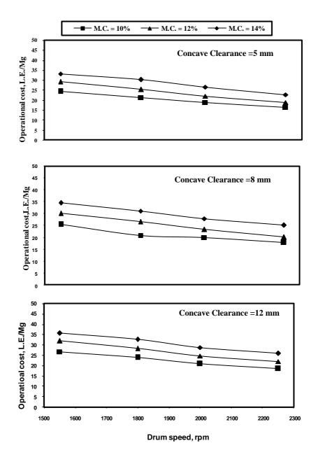
Fig.(12):Effect of drum speed on operational cost under different moisture contents and concave clearances at hammer thickness of 3mm.
