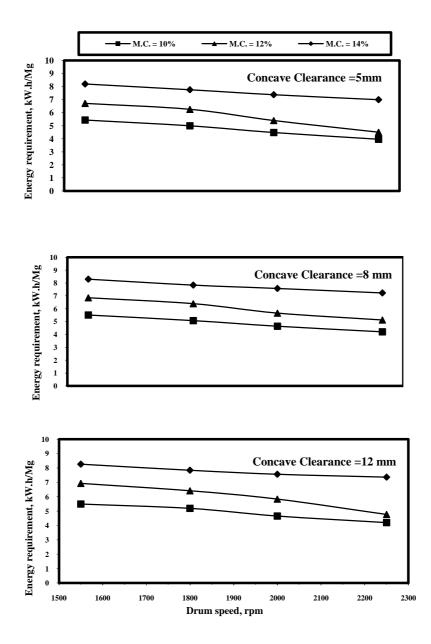
Fig.(8):Effect of drum speed on specific energy requirement under different moisture contents and concave clearances at hammer thickness of 1.5mm.
