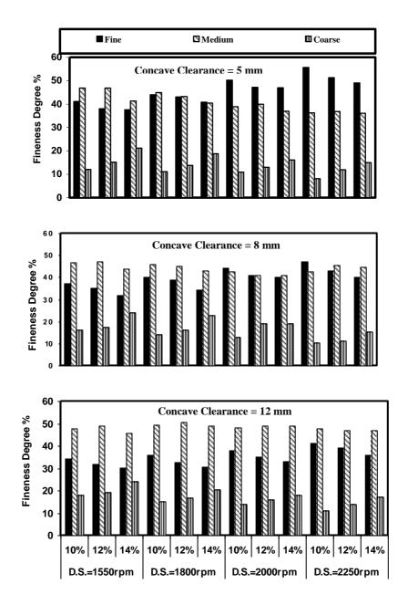
Fig.(7):Effect of drum speed on fineness degree under different moisture contents and concave clearances at hammer thickness of 5mm.
