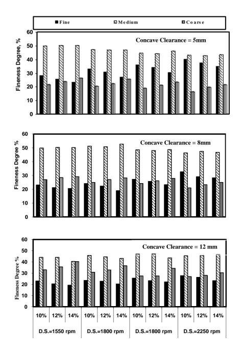
Fig.(5):Effect of drum speed on fineness degree under different moisture contents and concave clearances at hammer thickness of 1.5mm.
