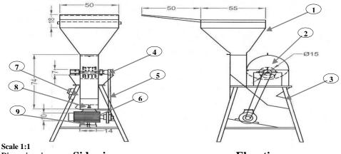
Dimensions in cm Side view Elevation Fig. (1): Elevation and side view of hammer mill prototype (1) Feed hopper, (2) Crushing chamber, (3) Outlet, (4) Pulleys, (5) Belt, (6) Motor, (7)
