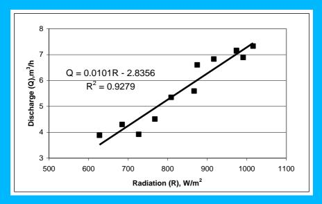
Fig. 6: Pump delivery correlated to solar radiation.
