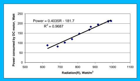
Fig. 7: DC motor power consumption (Watt) with different solar radiation values.
