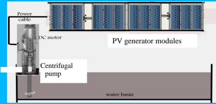
Fig. 3: Schematic drawing of pumping-set in site.
