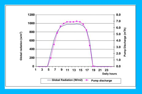
Fig. 8: Hourly average radiation (derived from Meteo-Norm software) and the computed pumping discharge for a selected month (June).
