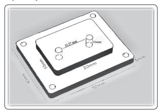
FIG (1) Diagrammatic measurements of the mold
