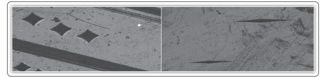
FIG (1) Group of Vickers indentations on composite and Knoop indentations on resin modified GIC at different loads and times.
