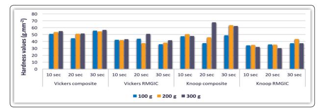
FIG (2) Comparative VHN and KHN values (Mean) of composite and RMGIC at different indentation loads and times.
