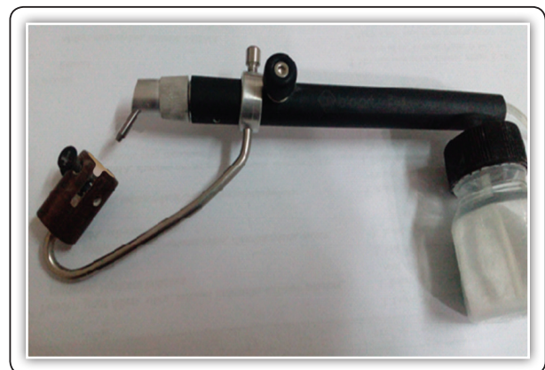
FIG (1) A photograph of a microblaster in the holder, nozzle perpendicular to zirconia specimen
