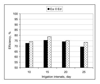
Fig. 1: The effect of irrigation intervals on the water application  $[E_a]$  and water distribution  $[E_d]$  efficiencies
