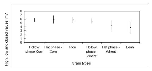
Fig. (6): The range and closed value of electrical reflection intensity for various grains using visible laser
