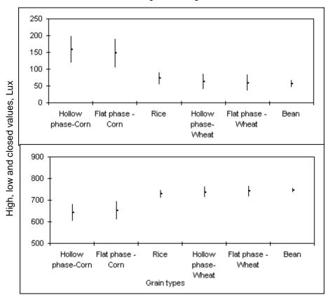
Fig. (7): The range and closed value of reflection and absorption intensity for various grains using visible laser
