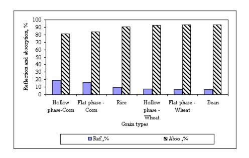
Fig. (4): Comparison between intensity of reflection and absorption percentages of various grains using visible laser.
