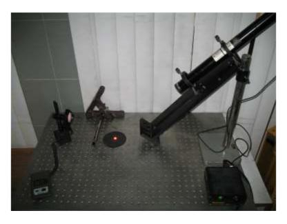
Fig. 1-a: Experimental setup for measuring optical properties of grains.
