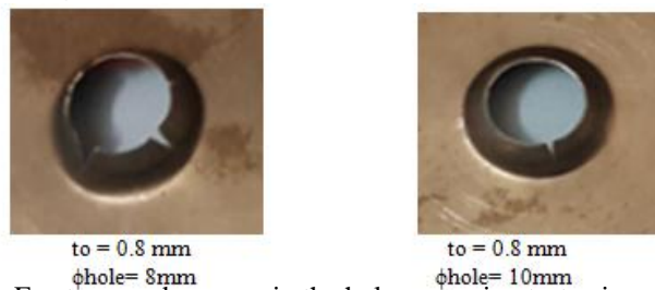
Fig. 12. Fracture modes occur in the hole expansion test using conical punch
